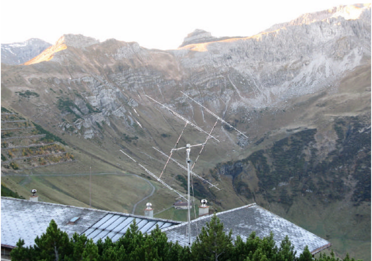
The 4 x 10 elements in HB0 at 2015 m ASL – yes, there is snow on the roof. (DK5EW)
